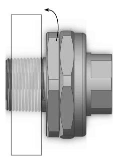
2. Slacken the nut (3) slightly to allow the conduit connector to turn relative to the entry item (1). Connect the conduit to the conduit connector and fully tighten.
