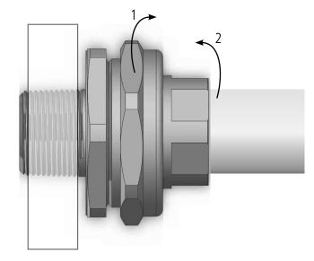
3. Fully tighten the nut (3) to ensure that the elements forming the serrated flamepath (2) are closely engaged.
