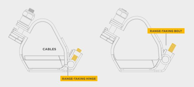
The Conqueror cable cleats are metallic cable cleats designed, constructed, and tested in accordance with the International Standard 'cable cleats for Electrical Installations' IEC 61914. The Conqueror cable cleat has been designed to restrain a large cable range take, and tested for exceptionally high short circuit conditions on cables held in trefoil application / formation, to ensure the securing and retention of cables without damage.
