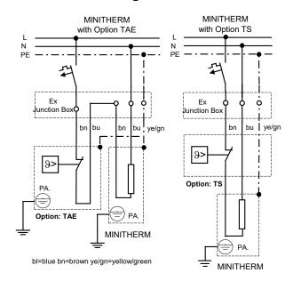
Connection Connection cable: silicone cable, notch and oil resistant, 3x1,5 mm<sup>2</sup>, 1m long. Other lengths available upon request (at an extra charge).
