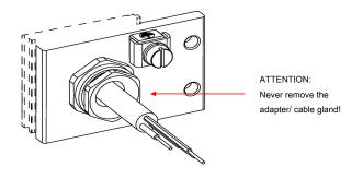
Illustration 3: Example heater with KLE connection
