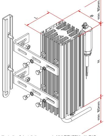
*Illustration 2:* Installation example MULTITHERM with TAE or TS and clearance
