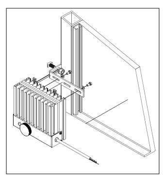
The mounting bracket and all shown bolts and nuts are supplied with the heater.
