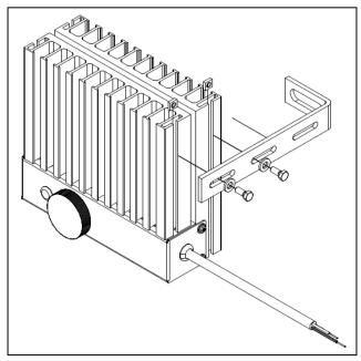
8.3 Attached to the C-Rail of an INTERTEC Protective Cabinet
